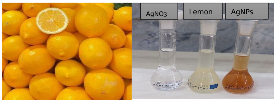
Figure 2: The change in color indicating the synthesis of AgNPs.
