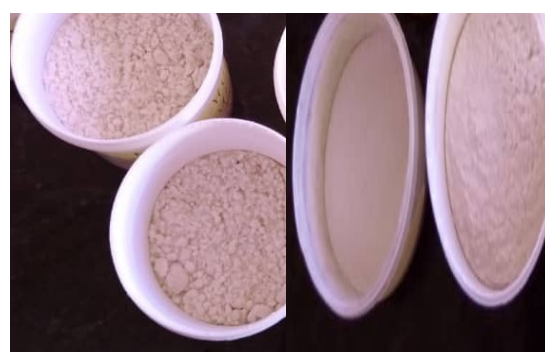
Figure 1: Cellulose extracted (left) and prepared microcrystalline cellulose (right).
