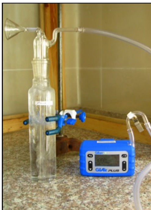
Figure 1: The air sample collection mechanism.
