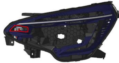
Fig.4 Location of FBL module in the headlamp
