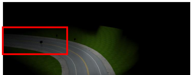
Fig.34. Simulation LB + V5 Cornering/Bending module
