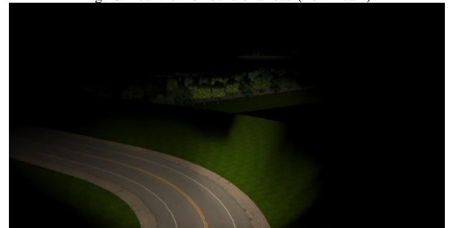
Fig.17. Real view on bend of a road (Low Beam+ Cornering/Bending)
