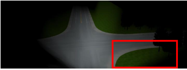
Fig.37. Simulation LB + V5 Cornering/Bending module on the corner
