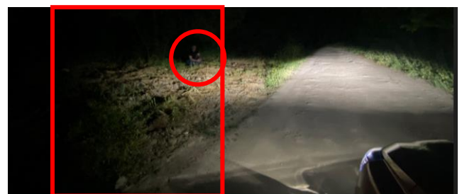
Fig.40. Night Drive test: low beam+ cornering/bending module
