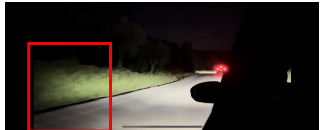
Fig.38. Night Drive test: low beam+ cornering/bending module
