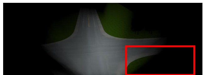
Fig.36. Simulation Low Beam distribution on the corner
