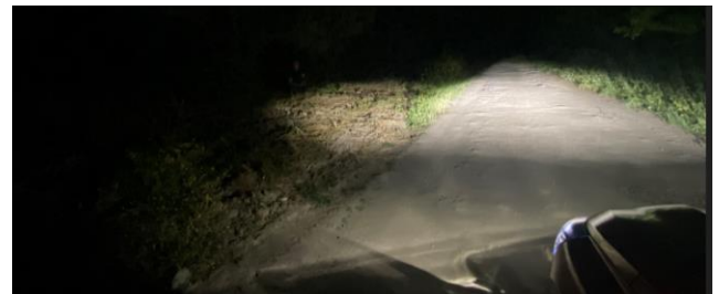
Fig.39. Night Drive test: only low beam
