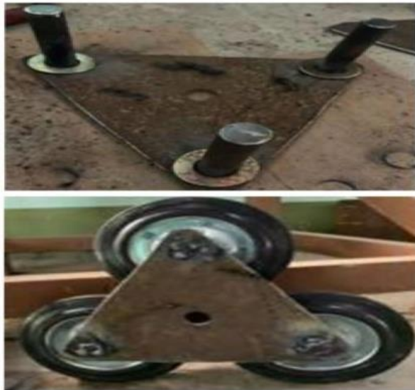
Figure 6. Pictorial view of the tri-stair wheel during fabrication.
