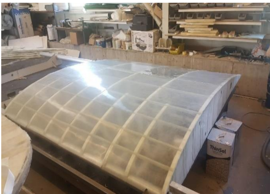
Figure 3. Construction of NACA4412 profile
