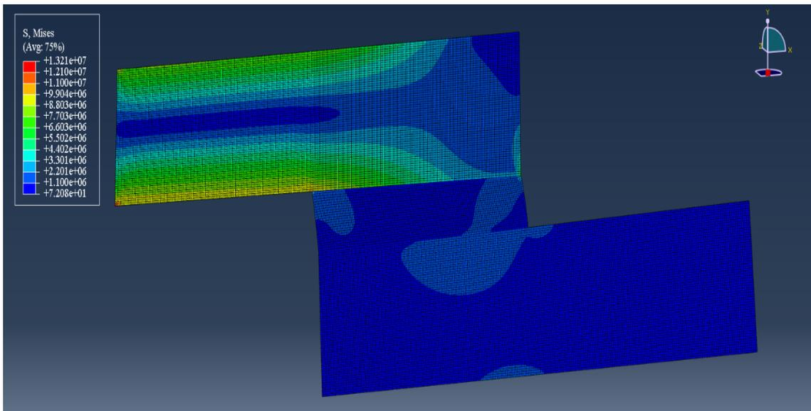
Fig. 13. Contour of Von Mises stress for adhesive I
