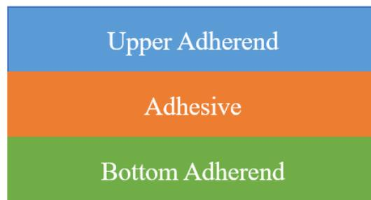
Fig. 1. General model of an adhesive bonded joint
