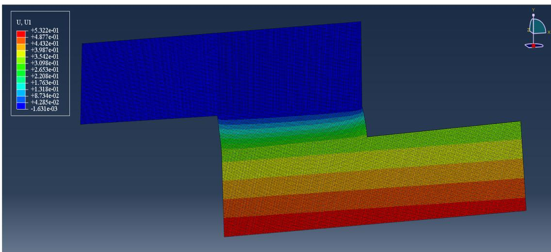
Fig. 11. Contour of displacement component  $u_1$  for adhesive I
