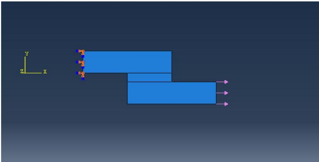
Fig. 7. Model showing boundary condition of the analysis
