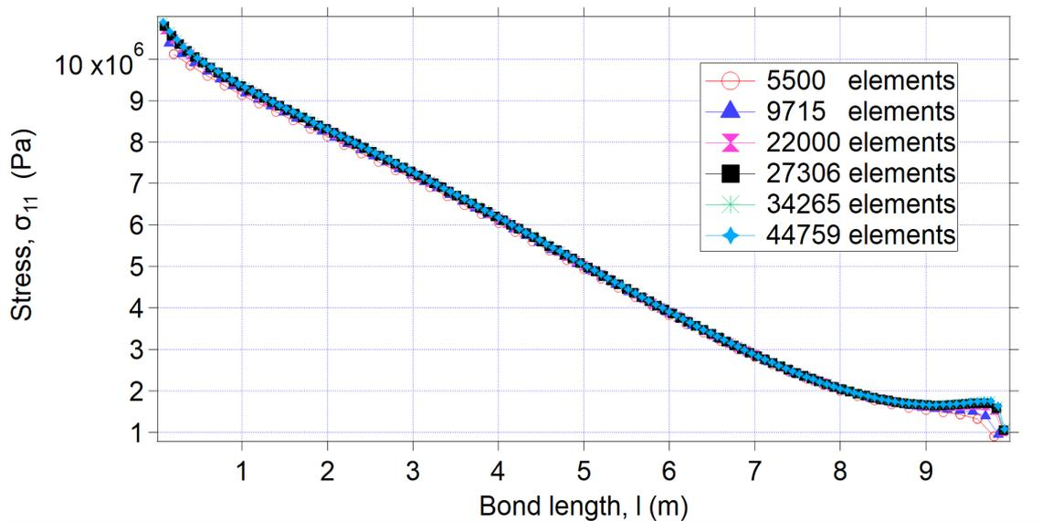
Fig. 6. Mesh sensitivity analysis of the model
