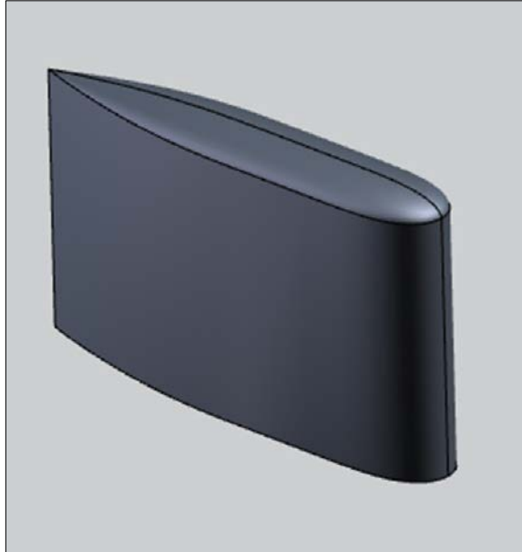
Figure 1. DARPA Suboff AFF8 submarine sail used in the case studies.
