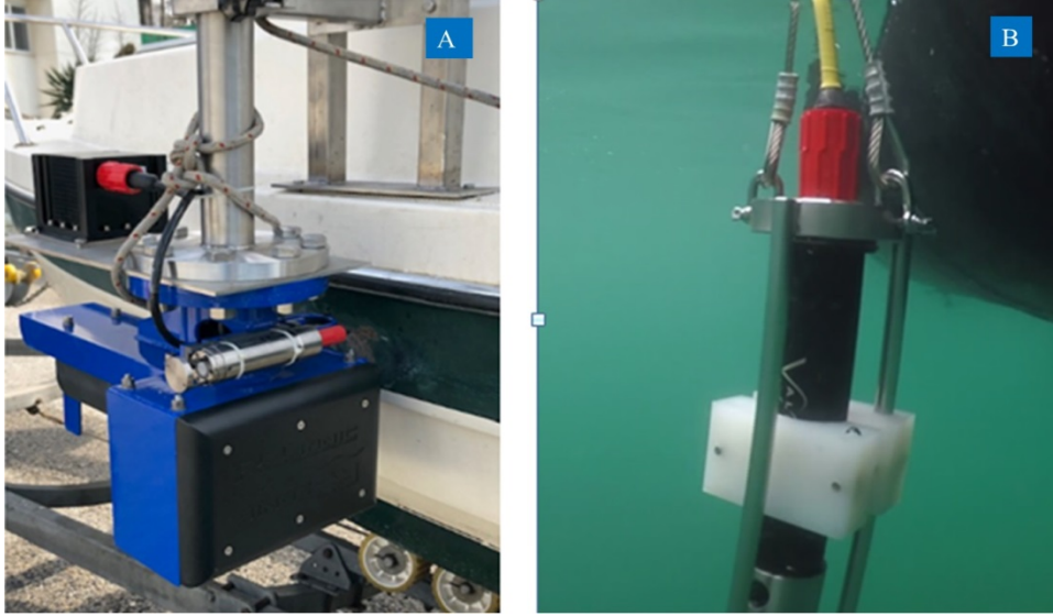
Figure 5. Equipment of R2SONIC 2022 400 Khz Multibeam Echosounder (A) and Valeport CTD (B).
