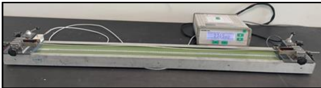
Figure 4. 4.02 mm alloy wire resistance measured after heat treatment
