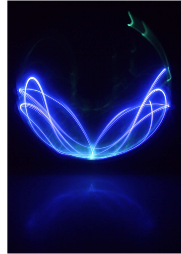
Figure 9 Double pendulum working with UV led placed on the tip of the second join. The image was taken with ISO 125 and a shutter speed of 4 seconds.
