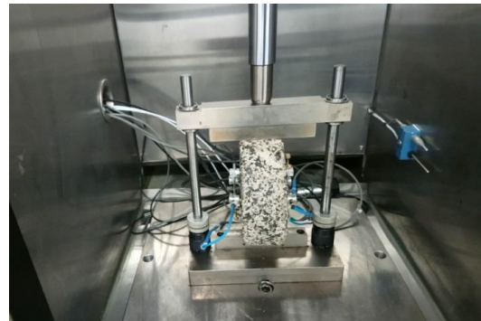
Figure 2. indirect tensile resilient modulus test application to foam bituminous mixture
