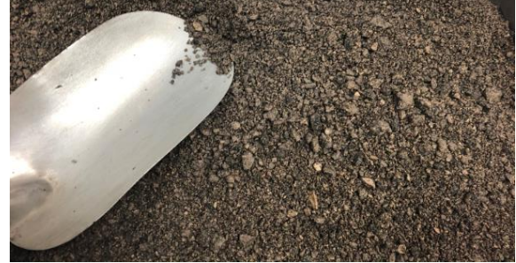
Figure 1. Foam bitumen stabilized material mixture produced with cement in uncompacted state [31]
