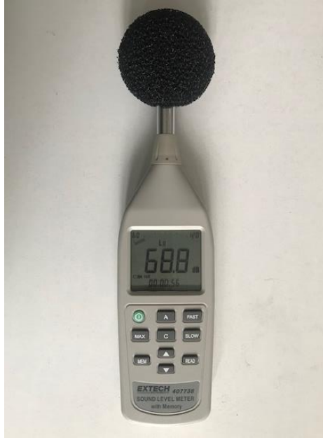
Figure 1. EXTECH SDL600 (Sound Level Meter) noise meter.
