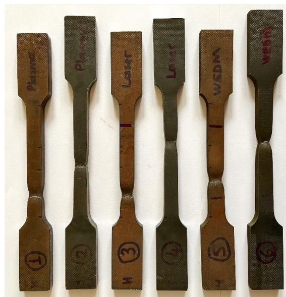
Fig 11. Fracture after tensile testing.
