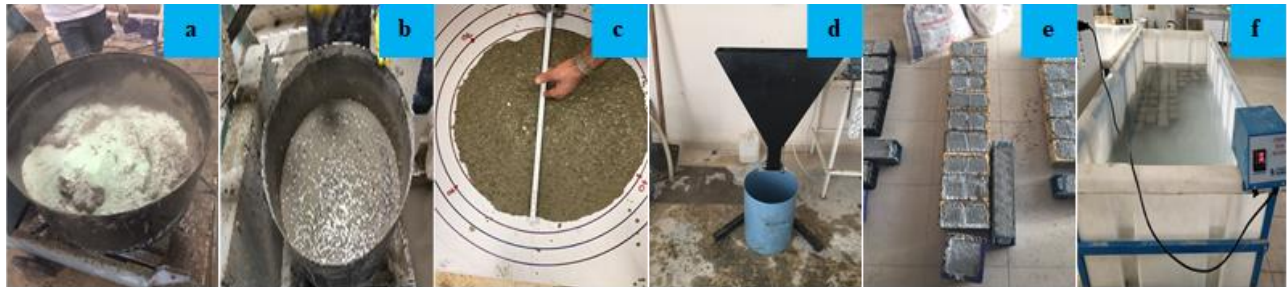
Figure 3. Laboratory fresh mixing, workability testing stages and curing.
