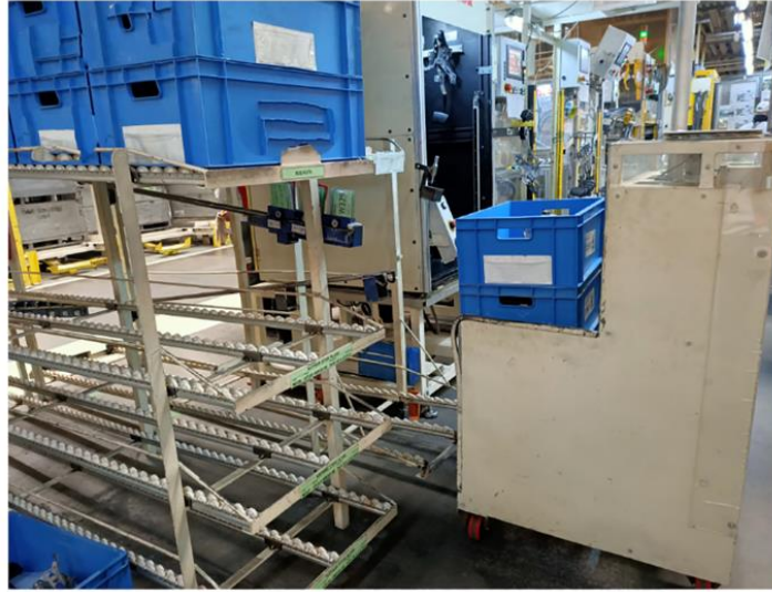
Figure 9. Karakuri and racking system integration
