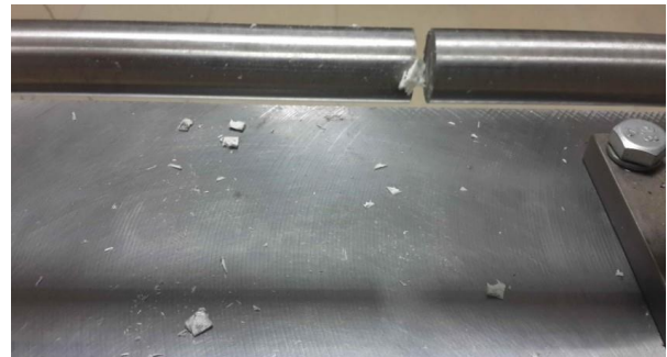
Figure 15. Disruption of the specimen under in-lane loading
