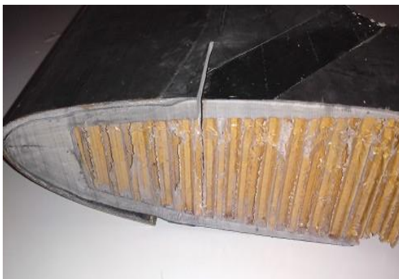
Figure 1. A real cross section from the helicopter blade.(outer surface; Carbon laminate, inner surface; glass laminate, core; Nomex honey comb)
