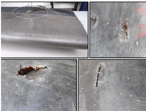
Figure 9. Damaged main rotor blade: Turkish Airforce Blade Repair Center
