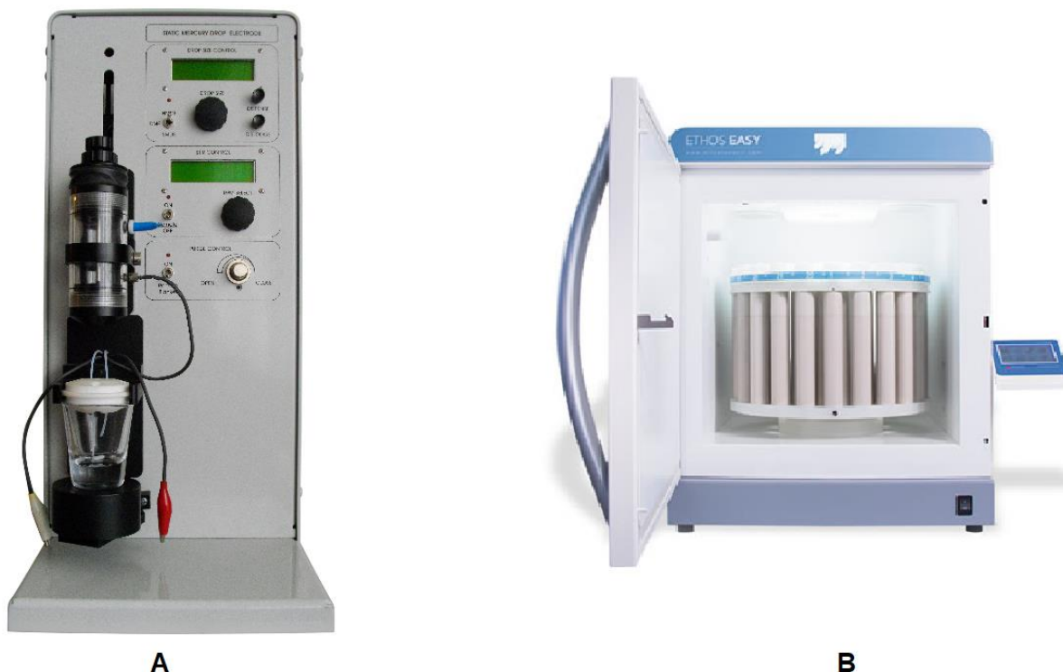
Figure 2. A) Polarography and B) microwave digestion device used during analyses
