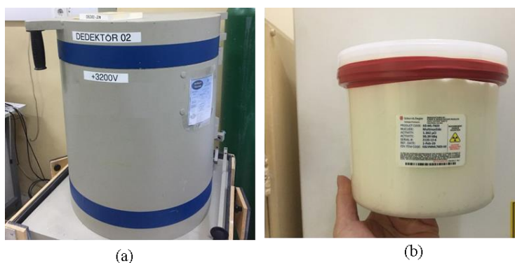
Figure 1. a) HPGe Detector, b) Marinelli beaker with 0.5 g/cc density used in the experiment
