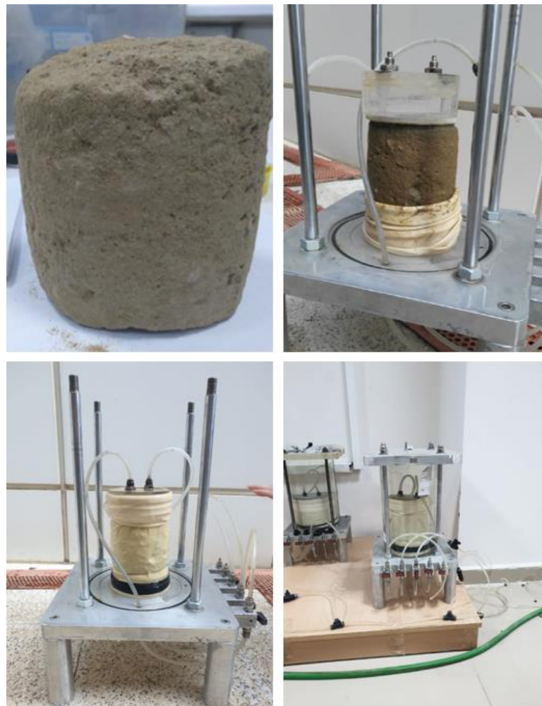
Figure 3. Setup and process of the hydraulic conductivity test
