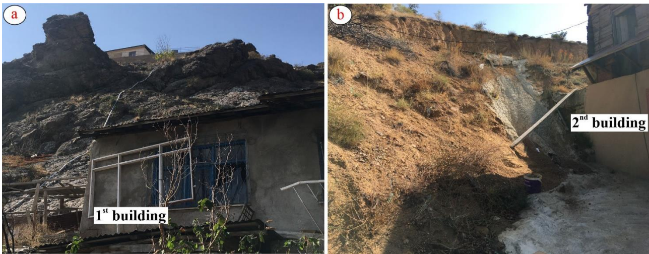
Figure 7. Field view of (a) the fissured and fractured andesite and (b) arenization of granite
