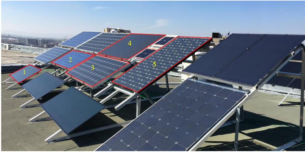
Figure 1. Configuration of ODTÜ-GÜNAM outdoor test facility (a) and tested modules – 1: CIS, 2: Poly-Si, 3: Mono-Si, 4: \mu\text{c-Si/a-Si} , 5: HIT (b)
