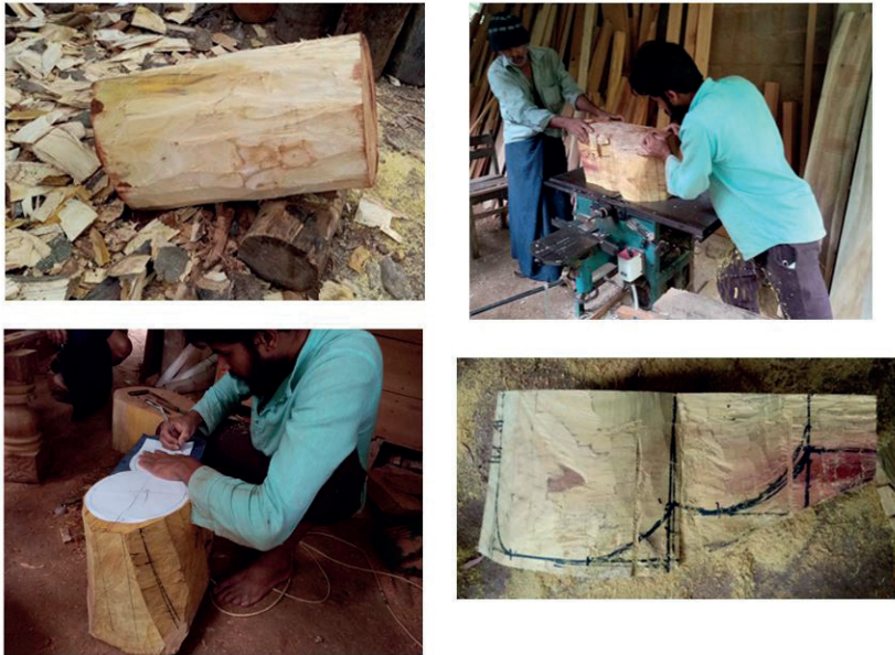
Figure 17. The part of the jackfruit wood used for the resonator (upper left); rough trimming the resonator (upper right); designing the resonator surface by marking the wood (bottom left); designing the side of the resonator by marking the wood (bottom right).
