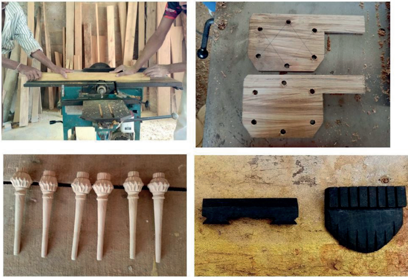
Figure 19. The neck (upper left), peg box (upper right), tuning pegs (bottom left), and the bridge and tailpiece (bottom right).
