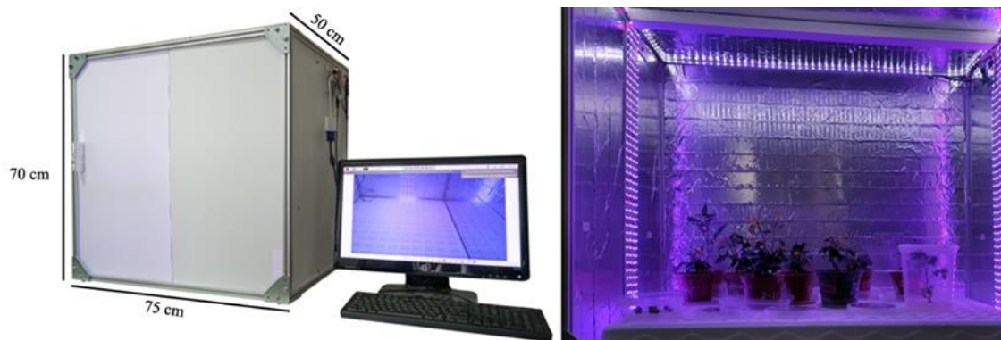
Figure 1. Exterior (on the left) and interior (on the right) of the custom-build growth chamber. The growth chamber was built in the specified dimensions (70x75x50cm) and was connected to a Raspberry Pi minicomputer. The minicomputer controls the photoperiod (20:4) through a simple 5V relay card with in-house built Python scripts. 12V blue and red LED as the light sources and were attached to either side of the growth chamber.
