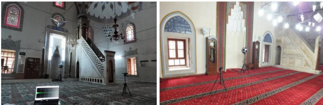
Figure 7 - The positions of sound sources and receiver points in the field measurements (left photo from the Yeni Mosque; right photo from the Sultan Mosque).
