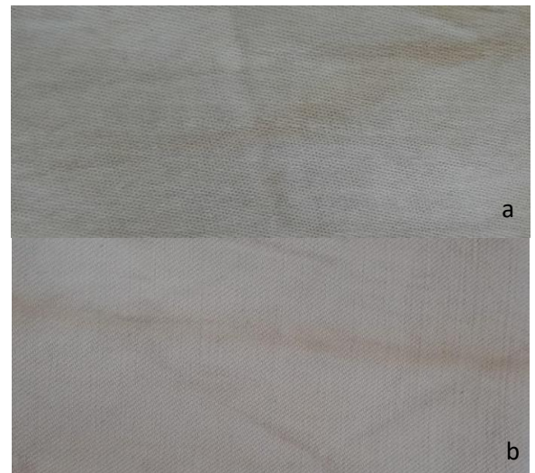
Figure 2. Product dyed with 1/1 product weight/coffee waste weight ratio and mordanted with a) quaternary ammonium compound, b) chitosan
