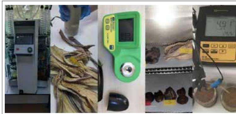
Figure 5. Equipment for analysis. A. used for oil determination; B. Spectropen colorimeter; C. Milwaukee MA871 refractometer device; D. Drying oven; E. pH meter. (Original)
