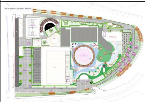
+10.80 Roof Plan Open to students, it has been converted into a terrace roof. An additional light band was added to the dome.
