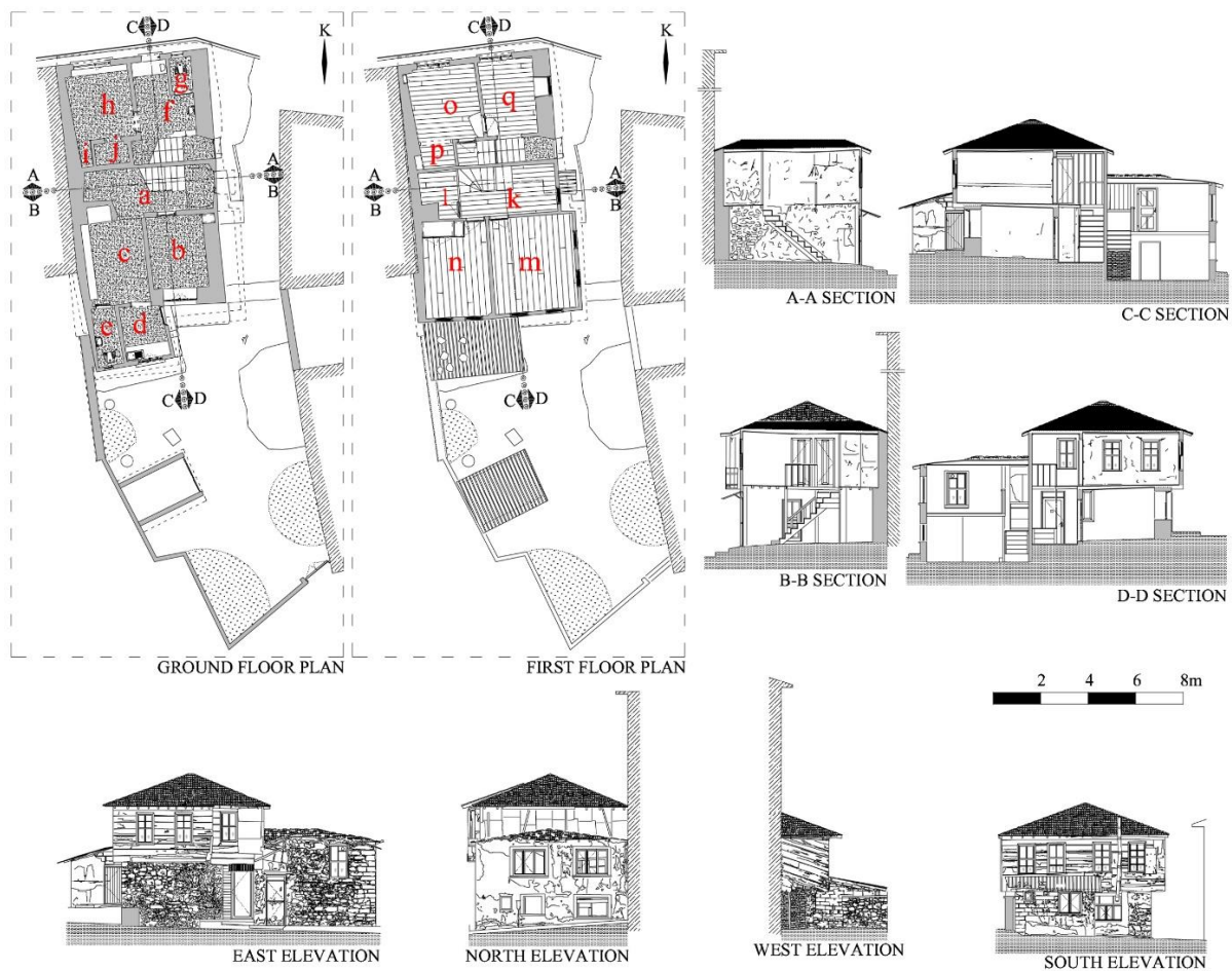
Figure 3. Measured drawing of Göksel Bey dwelling
