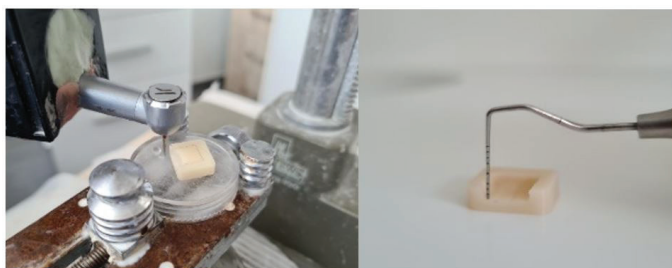
Figure 2. Cavity preparation with fine-grit cylindrical burs.
