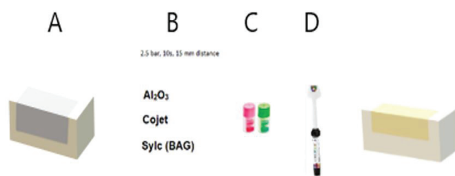
Figure 3. Preparation of the subgroups repaired with Omnichroma A) Cavity with dimensions of 8 \times 8 \times 2 mm, B) 2.5 bar; 10 s; surface preparation at a distance of 15 mm, C) Tokuyama Universal Bond application, D) Omnichroma composite application.
