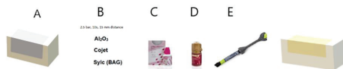
Figure 4. Preparation of the subgroups repaired with Essentia Universal A) Cavity with dimensions of 8 \times 8 \times 2 mm, B) 2.5 bar; 10 s; surface preparation at a distance of 15 mm, C) Multiprimer application D) G-Premio Bond application E) Essentia Universal composite application.
