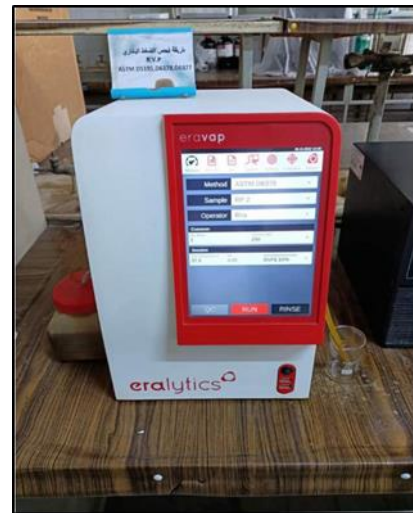
Figure 4: Reid vapor pressure apparatus.
