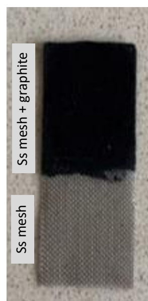
Figure 3. Stainless steel mesh + graphite electrode.
