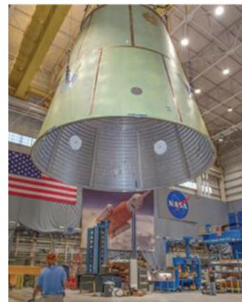
**Figure 10.** NASA SLS launch rocket produced by the FSW method [61]
