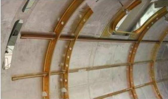
**Figure 11.** Demonstration of joined parts of the fuselage structure of Eclipse 500 private plane using FSW method [62]
