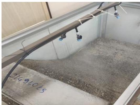
Figure 2. Precipitation mechanism
