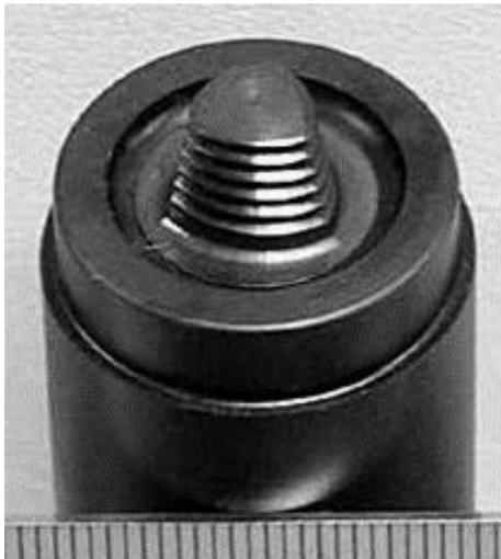
Figure 6. Trivex tool, designed by TWI [25]
