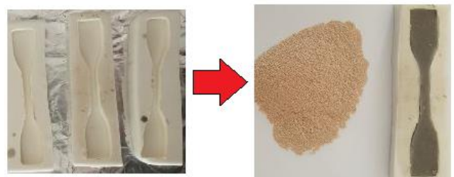
Figure 2. Polyester composite production scheme
