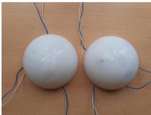
Figure 4. The prepared breast phantoms with buried different resistors as a tumor structure.
