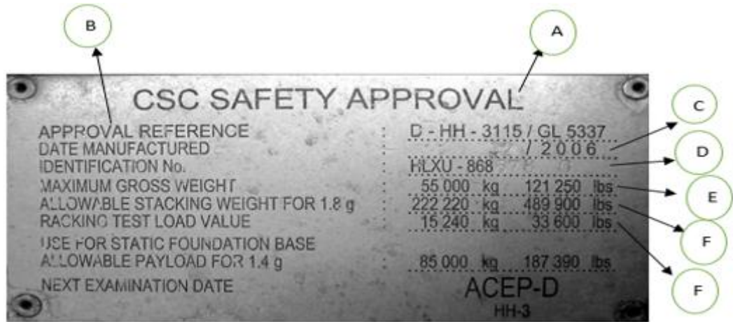
Figure 1. Safety Approval Plates
