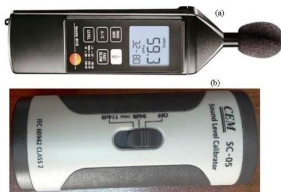
Figure 1. (a) The photographs of the Testo 815 decibelmeter, and (b) CEM SC-05 sound level calibrator devices.
