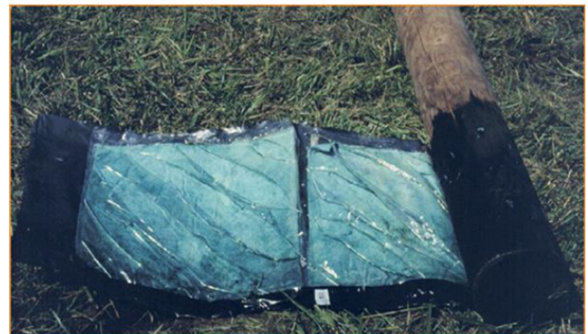
Figure 2. Example of a self-contained copper/boron preservative bandage
