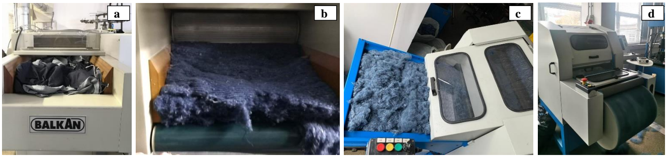
Figure 1. (a) Feeding and (b) output unit of rag pulling machine, (c) feeding and (d) output unit of carding machine
