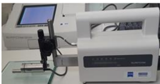
Figure 2. Surface roughness tester (Surfcom 130 A)
