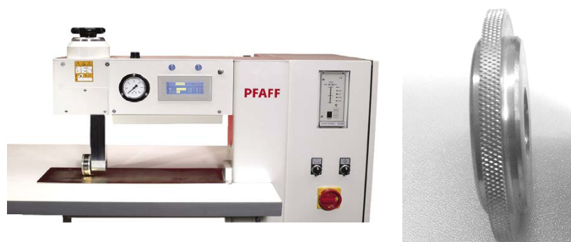
Figure 1. (a) Pfaff 8310 Seamsonic Ultrasonic Sewing Machine, (b) The roller
