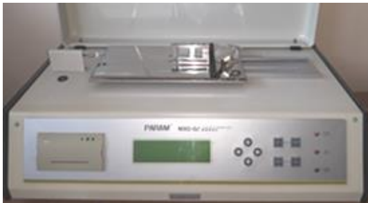
Figure 1. Friction coefficient tester (Labthink Param MXD-02)
