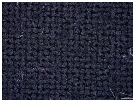
Figure 15. Surface images of F-7 A) Untreated B) 40 g/l PVCL treated
