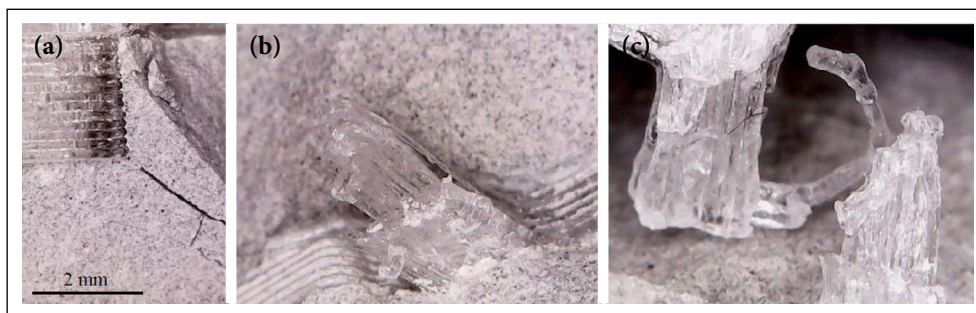
Figure 9. (a) Micro-cracking of the matrix, (b) Slipping of layers, (c) Rupture of the reinforcement.
