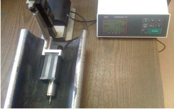
Figure 2 Profilometer device measuring roughness on painted sheet surface
