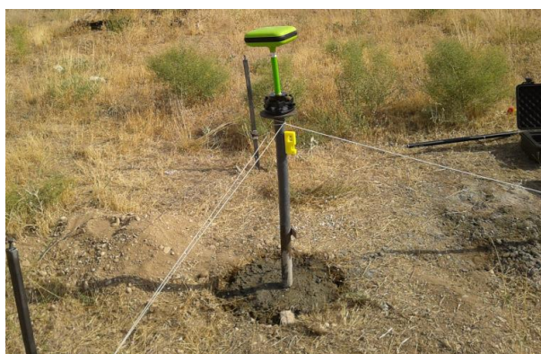
Figure 1 Fixed station established in work area
