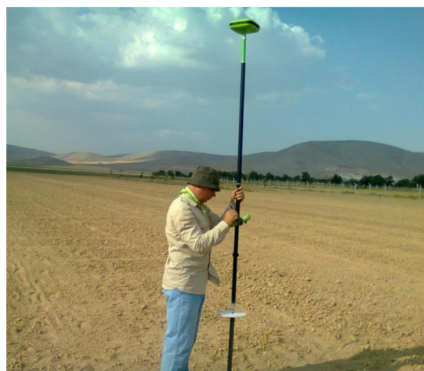
Figure 3 Coordinate points with a roving GPS tool
