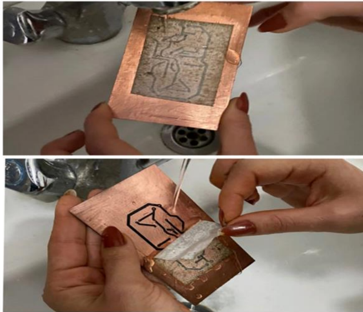
Figure 4. Separation of transfer paper over pertinax
