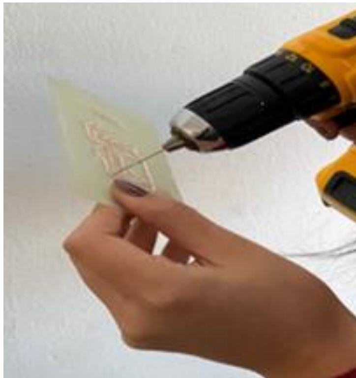
Figure 6. Opening the slots of the components that will be mounted on the circuit
