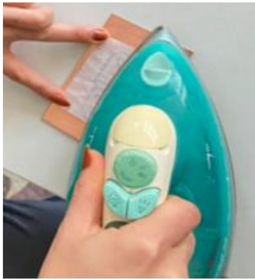
Figure 3. Passing the circuit to the pertinax with the help of heat
