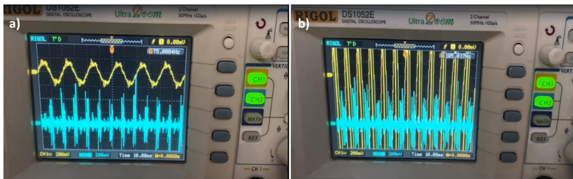
Figure 10. a) Regularly generated sine waves of Fizyopol brand TENS and BUSER TENS. b) Oscilloscope image when Fizyopol TENS device and BUSER TENS device pulse
