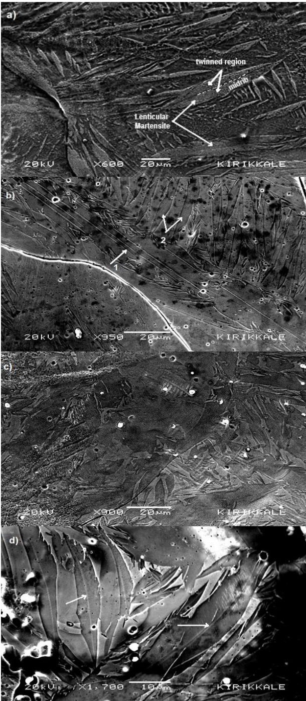
Figure 2. Thermally induced b.c.c. ( \alpha' ) martensite structures; (a-b) lath and lenticular martensite in Fe-30wt.%Ni-2.6wt.%Mo-0.8wt.%Co, (c-d) massive and lenticular martensite in Fe-30wt.%Ni-2.6wt.%Mo-1.8wt.%Co.
