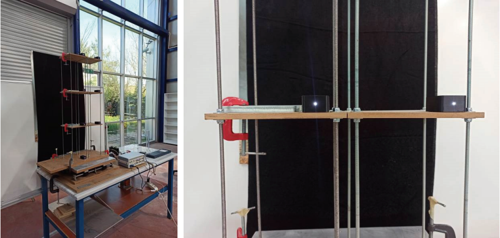
Figure 3 - General view of the experimental setup (left) and LED markers placed on the floors (right)
