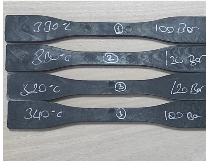
Figure 2. Tensile test specimens for PPS
