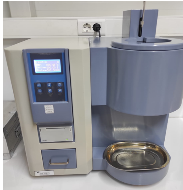
Figure 7. Melt flow index test of polymers
