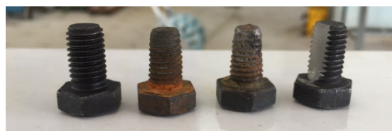
Figure 4. Accelerated and artificial corrosion of the bolts
