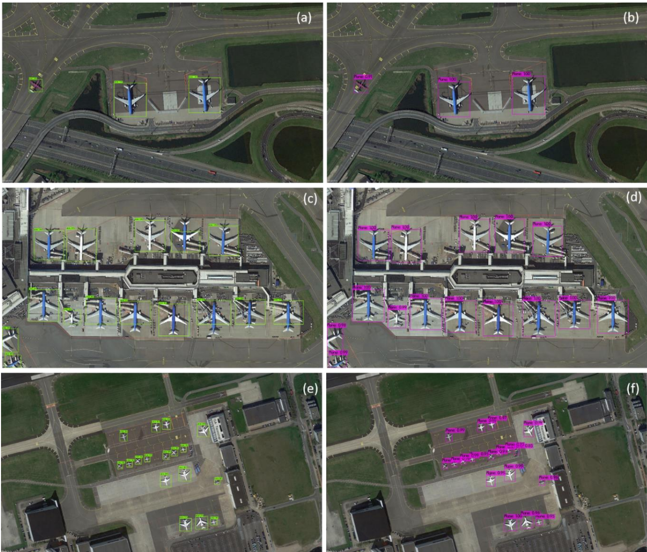
Figure 2. Prediction results of Faster R-CNN (green) and YOLOv4 (purple) from Amsterdam Schiphol Airport
