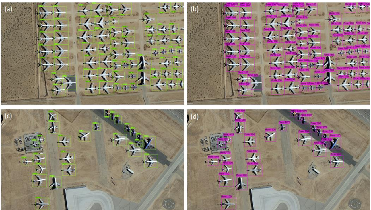
Figure 7. Prediction results of Faster R-CNN (green) and YOLOv4 (purple) from a plane graveyard
