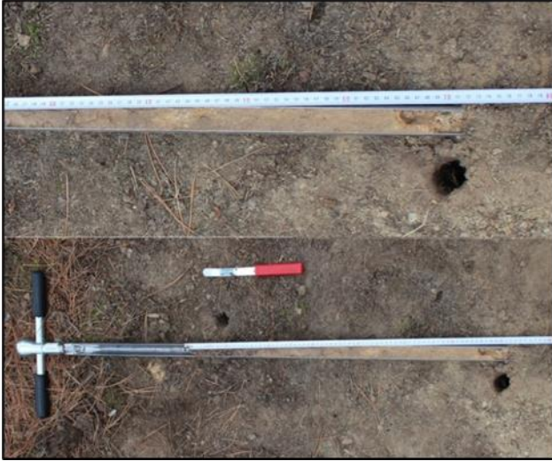
Figure 2. A view from sampling with a 100cm auger to determine soil depth.
