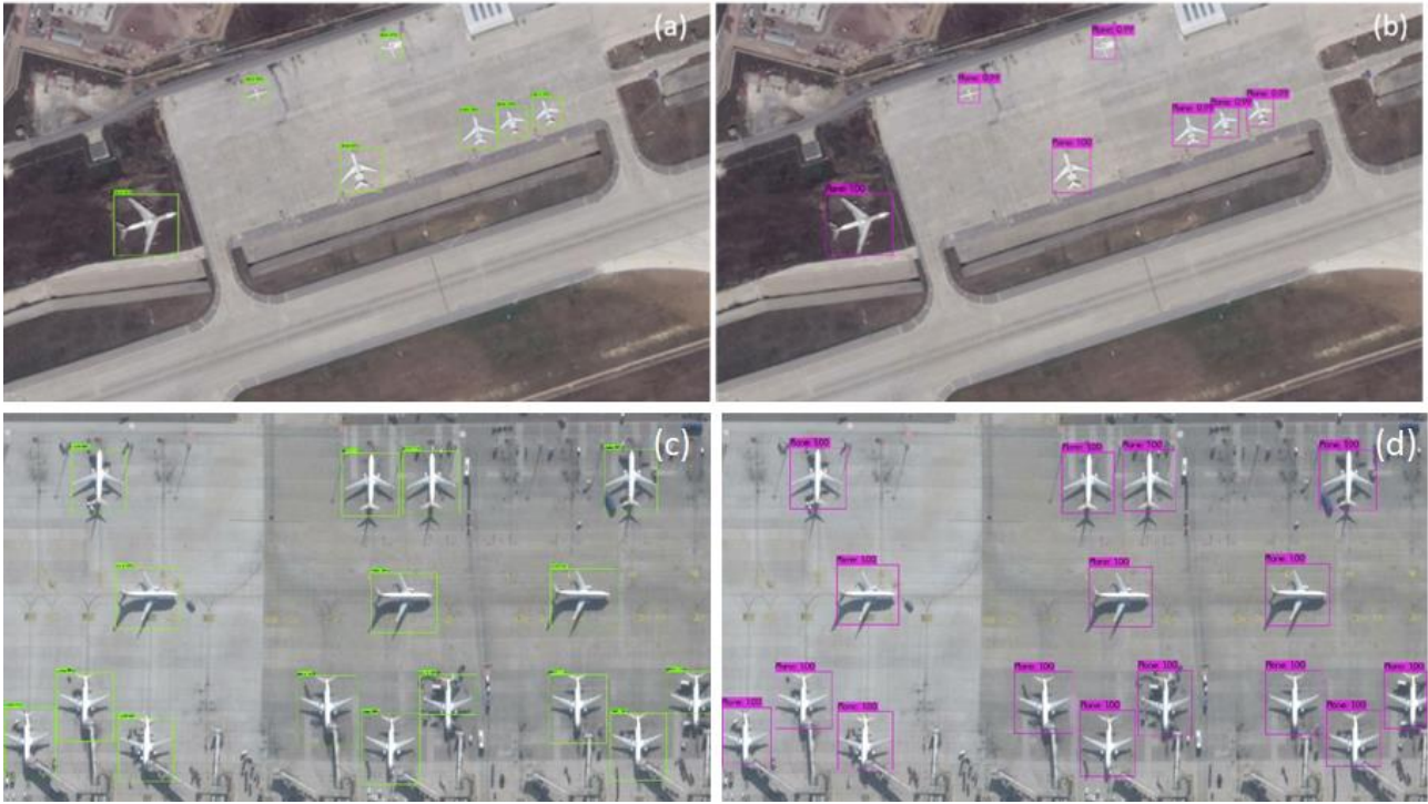
Figure 3. Prediction results of Faster R-CNN (green) and YOLOv4 (purple) from Istanbul Sabiha Gokcen Airport
