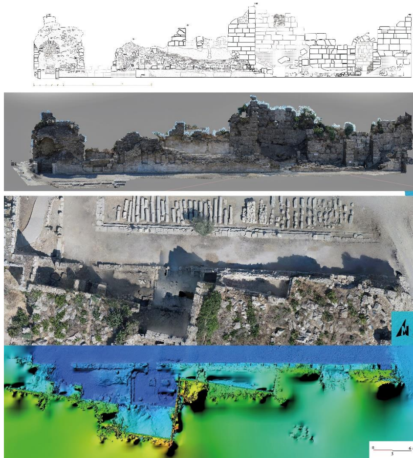
Figure 5. Documentation samples prepared with the Agisoft Metashape program. From below: The topographic view of the South Stoa, the photograph of the back wall of the stoa without perspective, and the technical drawing obtained from Agisoft data
