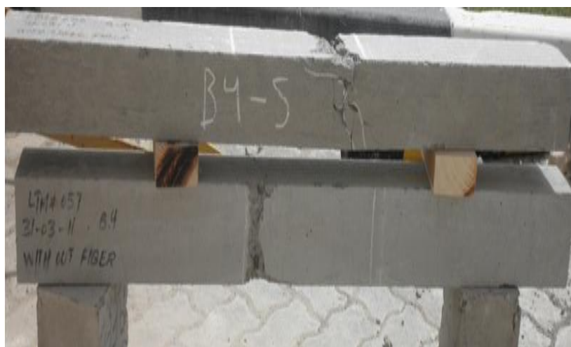
Figure 5: Failure mode under static load, for the steel fibers, reinforced concrete beam, B4 – S, and control beam B4 – C
