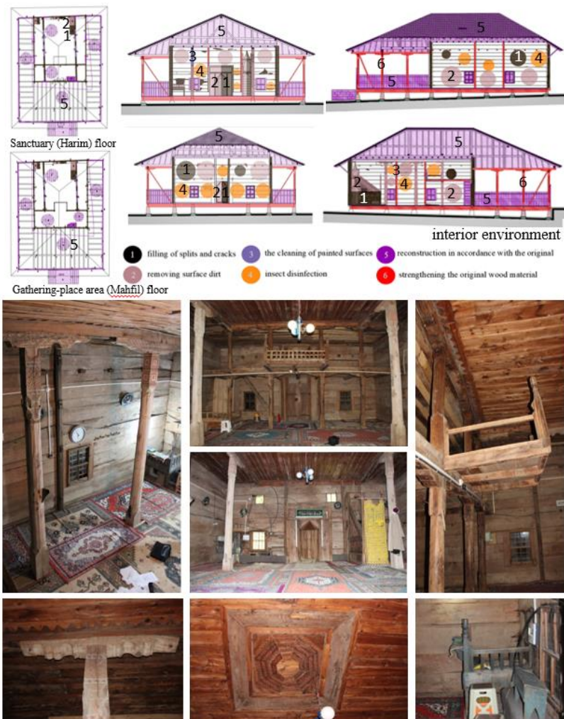
Figure 10. Deformation and interventions in wooden material in Ordu village mosque; sanctuary, gathering place and wooden items
