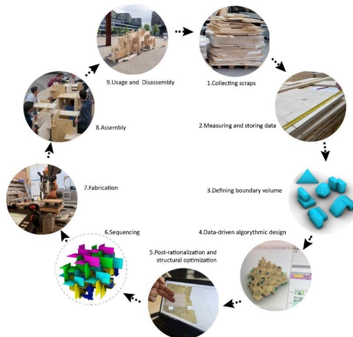
Figure 2. Proposed design, fabrication and assembly process in steps
