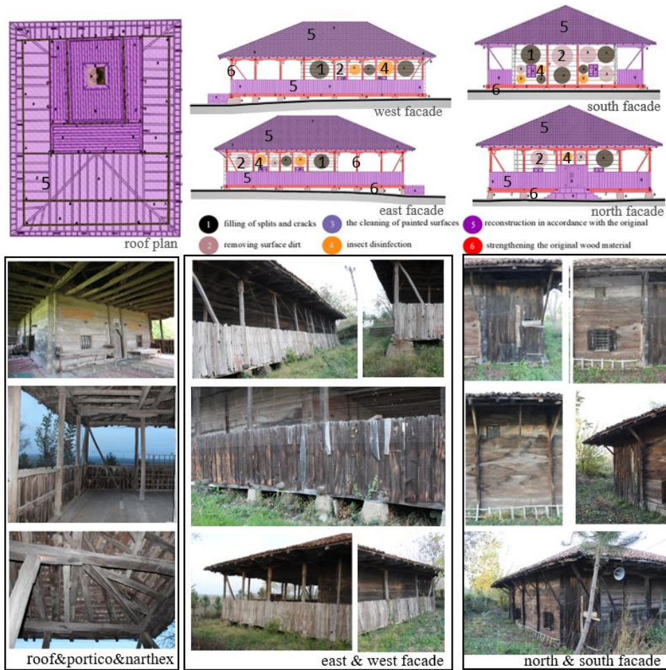
Figure 9. Deformations and interventions in wooden material in Ordu village mosque; roof, narthex, portico and façade
