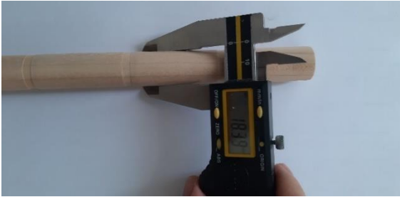
Figure 4. Measurement of test specimens' diameters with the caliper.
