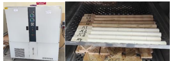
Figure 2. The position of the experimental specimens in the air-conditioned cabinet
