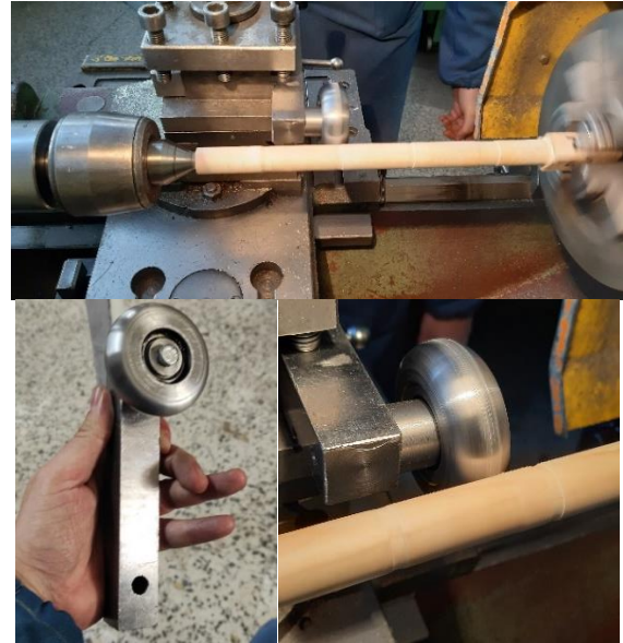
Figure 5. Densification of cylindrical parts with a spinning roller.
