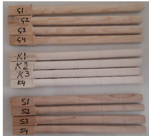
Figure 1. Test specimens before densification
