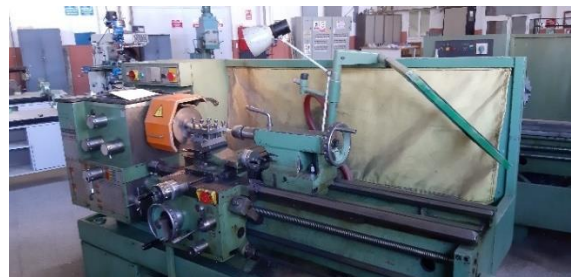
Figure 6. TOS GALANTA SUIL 40A lathe.
