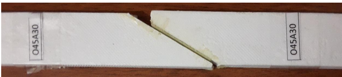
Fig. 10. Demonstration of the test specimens with the optimized scarf angle of 30°.
