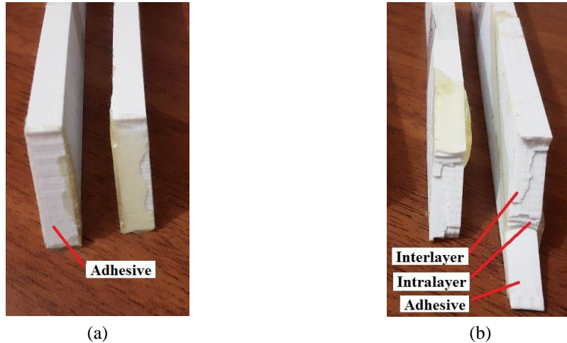
Fig.8 Debonding surfaces of two selected joints, (a) O0A60, and (b) O45A15. Different types of failure including Adhesive and Adherend (Interlayer and Intralayer) were labeled in the figures.
