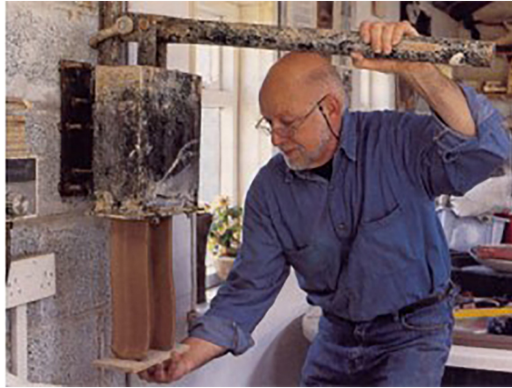
Görsel 3. Manuel Çamur Ekstrüzyonu. Carter ve Norton, (2013), Ceramic Materials: Science and Engineering SpringerLink: Bücher, s. 432.
