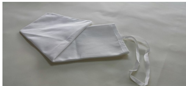
Figure 3: Electroplating anode bag used in Cu and Ni coating.
