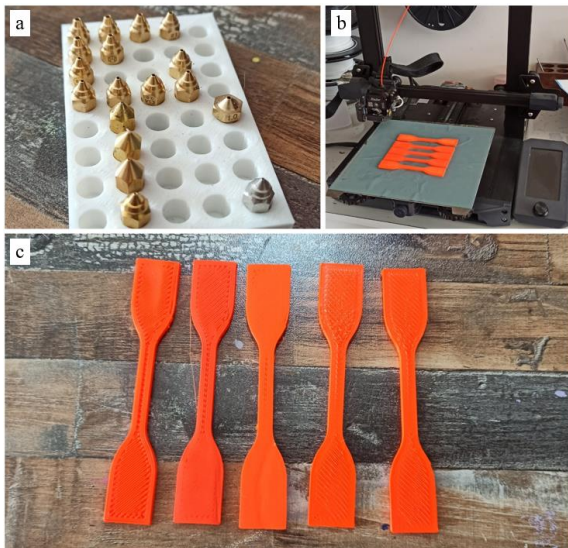
Figure 2. (a) Nozzles of different diameters used in printing, (b) Ender 3 S1 3D printer and (c) Produced the tensile sample of 3D-printed parts according to ASTM-Type IV.
