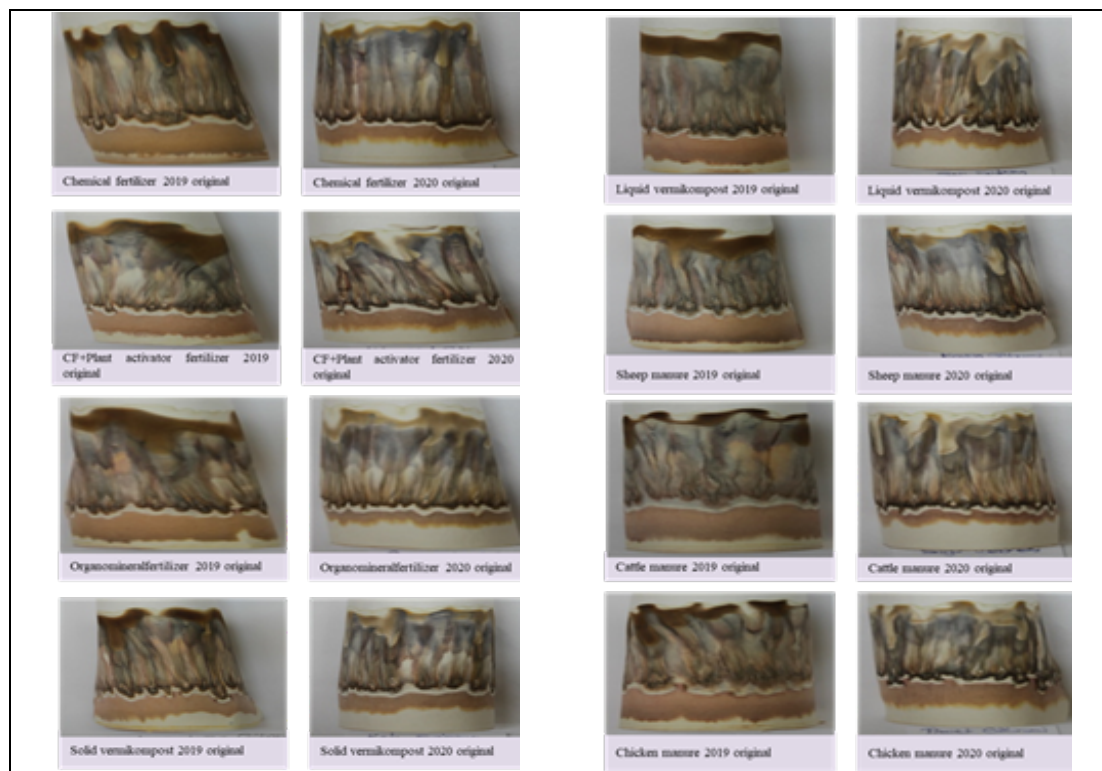
Figure 6. Rising picture chromatogram of some frozen tomato samples in 2019 and 2020 (100% frozen tomatoes, 0.5% silver nitrate, 0.5% ferrous sulfate solution).
