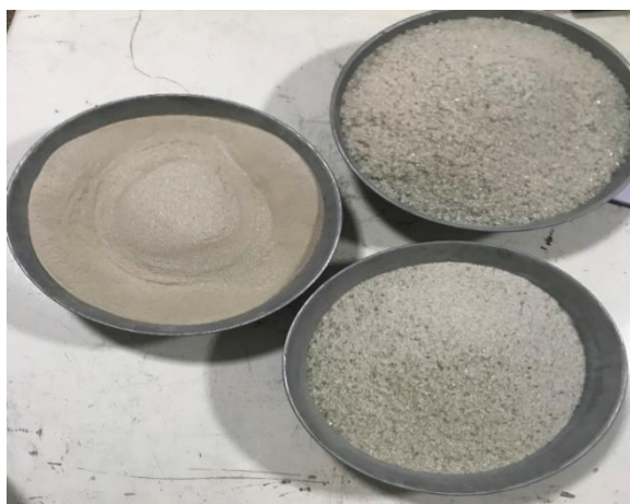
Figure 2: Sieved glass powder for cement and sand
